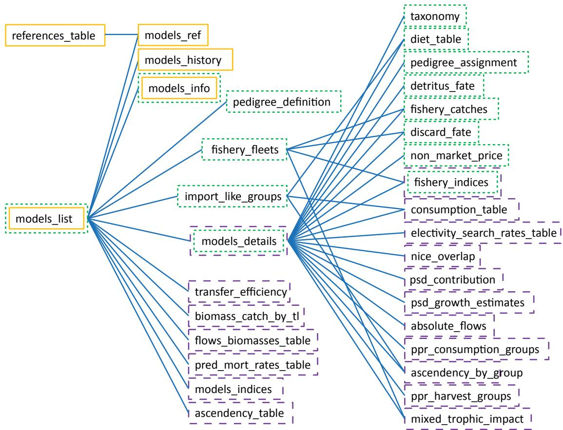
**Figure 8.** Diagram of tables relations (orange solid contours indicate tables containing metadata, green dotted ones tables containing EwE inputs, and purple dashed ones tables containing EwE outputs).
