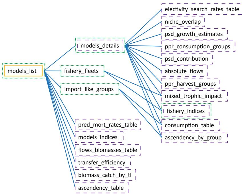
**Figure 5.** Relation diagram of the EwE input tables (orange solid contours indicate tables containing metadata, green dotted ones tables containing EwE inputs, and purple dashed ones tables containing EwE outputs).
