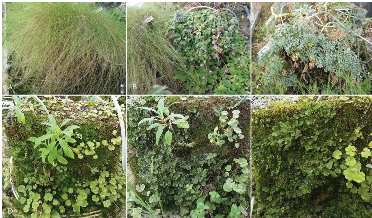
Fig. 3. Interior trials 1, 2&3: Top row: Long-term results of 1 st and 2 nd series in 2018. A: 2 nd series block showing Lolium perenne , and Festuca rubra (2018). B: 2 nd series test block showing Centranthus ruber and Cymbalaria muralis taking over but Ruta graveolens peeking through (2018). C: 1 st series test block (Metakaolin formula with soil substrate) after three years (2018) with Ruta graveolens taken over (note: the Ruta Graveolens appeared one year after seeding). Bottom row: Mid-term results of 3 rd series of temporal trials (2017). D: Seeded one week after casting. E: Seeded two weeks after casting. F: Seeded three weeks after casting. Photos by Fabienne Mathis and Vegepolys.
