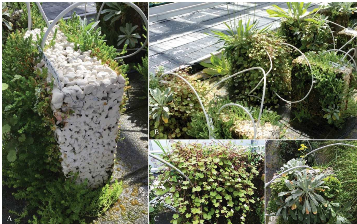
Fig. 2. Interior trials 1&2: A: 2 nd series results and the prodigious Sedum acre ( Cymbalaria muralis showing) on a white cement/Metakaolin/limestone filler test block with Rockwool seeded-substrate (2016). B: wider view of 1 st and 2 nd series trials in the Angers greenhouse (2016). C: Mid-term results (2017) showing a test block of the cement formula with soil substrate and Cymbalaria muralis taking over. D: 1 st series test block of the cement formula with soil substrate and cement added to soil and Aurinia saxatilis dominating. Photos by Benjamin Riley.
