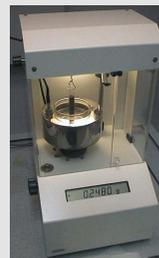
**Figure 2.** Instrument for determining contact angles on porous material (e.g. substrate)
