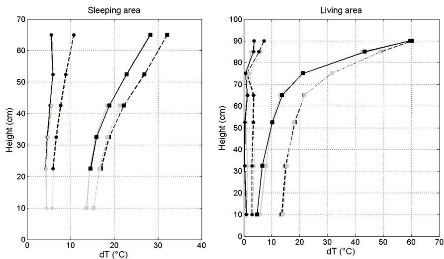
**Figure 6 :** Thermal gradients within the sleeping area (left) and living area (right) for forced and mixed convection ('o' and '□' symbol respectively) for configuration with mosquitoes closed (dotted line) and open (line) for the reduced scale model.
