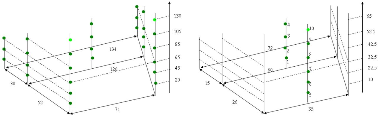
**Figure 4 :** Position of the thermocouples in the sleeping area of the full scale model (left) and reduced scale model (right)
