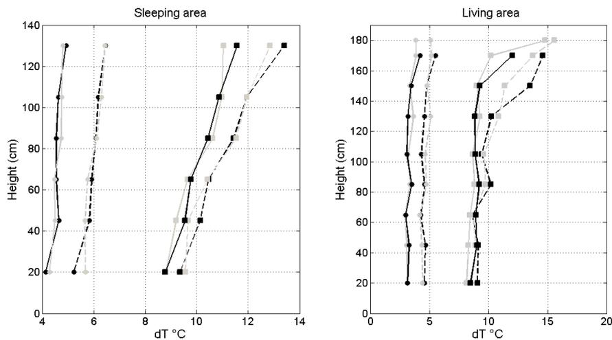
**Figure 5 :** Thermal gradients within the sleeping area (left) and living area (right) for forced and mixed convection ('o' and '□' symbol respectively) for configuration with mosquitoes closed (dotted line) and open (line) for the full scale model.
