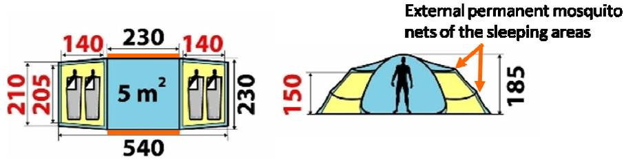
**Figure 1 :** Description of the tent at full scale with one living area (blue) and two sleeping areas (yellow). The indicative position of the mosquito net is coloured in orange in living and sleeping area
