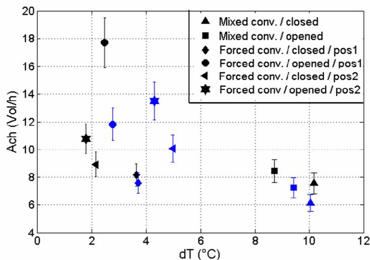
**Figure 7 :** Representation of air change rate (Ach) measured on both scales. Same symbol are used for each configuration, blue colour is used for the full scale model and black colour for the reduced scale model. In the legend, 'conv' stands for convection, pos1 to a stream-wise position of the tent and pos2 to a span-wise position of the tent
