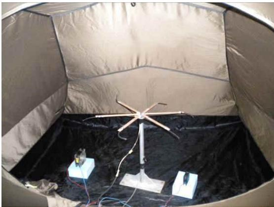
**Figure 2:** *experimental setup of the tracer gas technique in the sleeping area*
